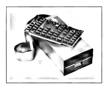
**POWER:** The power requirement of the controller board is .7 amps at 8V. The power requirements for a single disk drive are:
