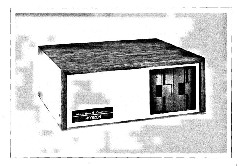
The **HORIZON** Computer is a complete, high-performance microcomputer system with integrated floppy disk memory. To begin programming in North Star extended disk BASIC, merely plug in a CRT or hard-copy terminal. Operating a HORIZON is simple: there is only an on/off switch and a restart button. The North Star software is loaded from diskette within seconds after power-on.
