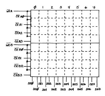
ARRAY CONSISTS OF 64 (4KXI) STATIC RAMS STATLAR TO MM5257-OR SM0030B U.18 – U.81
