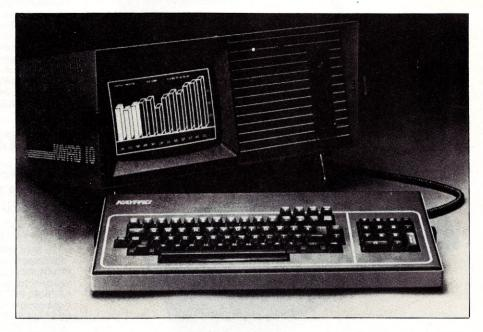
on the Kaypro 10 it automatically logs you onto the hard disk; before power off, you must remember to type SAFETY.
