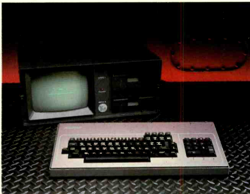
The Kaypro 4 Plus 88 features an Intel 8088 and an added 256K.
