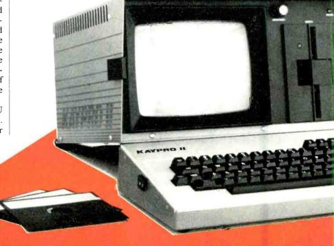
1920 characters at one time. A front-panel BRIGHTNESS control is provided to adjust the display as desired, while the 25-MHz video monitor bandwidth enhances viewing of the display. Although the computer has 64K of RAM, a bank separate from the user-RAM area has the 2K system ROM and the 2K video display RAM.
