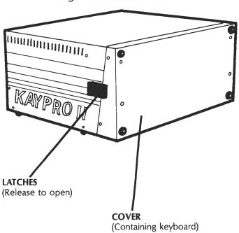
First, set the computer on the work surface with its blue base in front. (This is actually the "cover" that contains the keyboard.)
