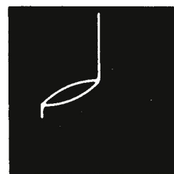
Transistor base-emitter paralleled to 1 \mu F + 680 \Omega
