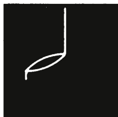
B-E with 1\mu\text{F} + 680\Omega
